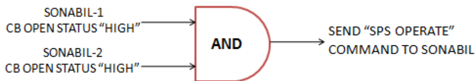
Fig 34: SPS Logic to be configured at Balipara end
